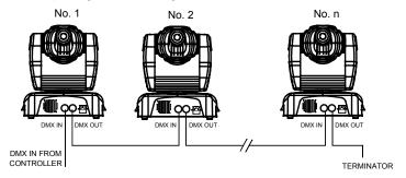
Connect the controller's output to the first fixture's input, and connect the first fixture's output to the second fixture's input. The rest may be deduced by analogy. Eventually connect the last fixture's output to a DMX terminator as shown in the figure above.
