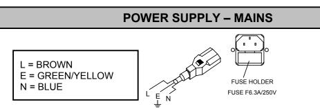
Use the plug provided to connect the mains power to the projector paying attention to the voltage and frequency marked on the panel of the projector. It is recommended that each projector is supplied separately so that they may be individually switched on and off.
