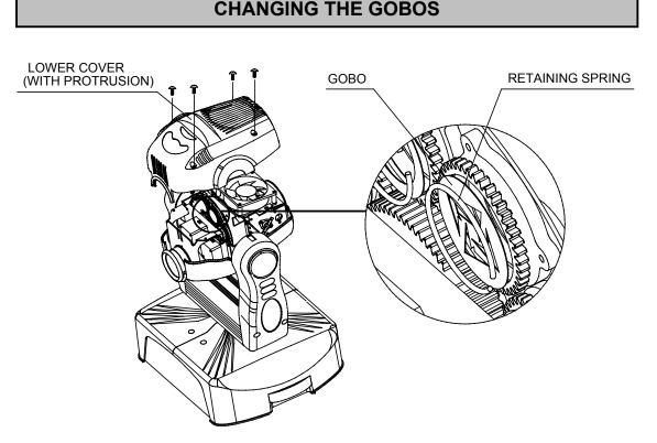
Carefully lift off the lower cover by undoing the 4 screws. (Note: the lower cover has an obvious protrusion on the surface, which is different from the upper cover.)
