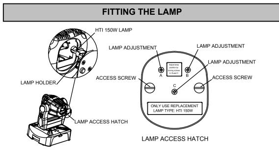
Open the lamp access hatch at the rear of the projector by undoing the 2 access screws as shown above.
